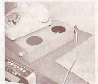
The adaptor box (above) enables messages typed on the T.T.Y. (below) to be sent by phone.
